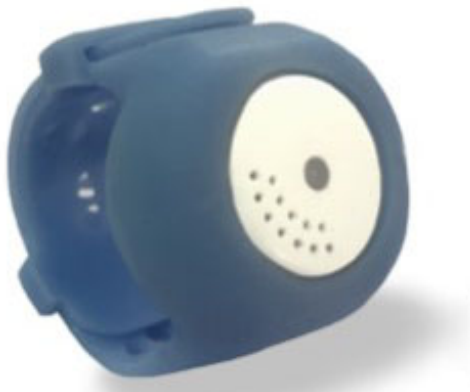
Web Fig. 1 BEMPU bracelet; a hypothermia monitoring device.
